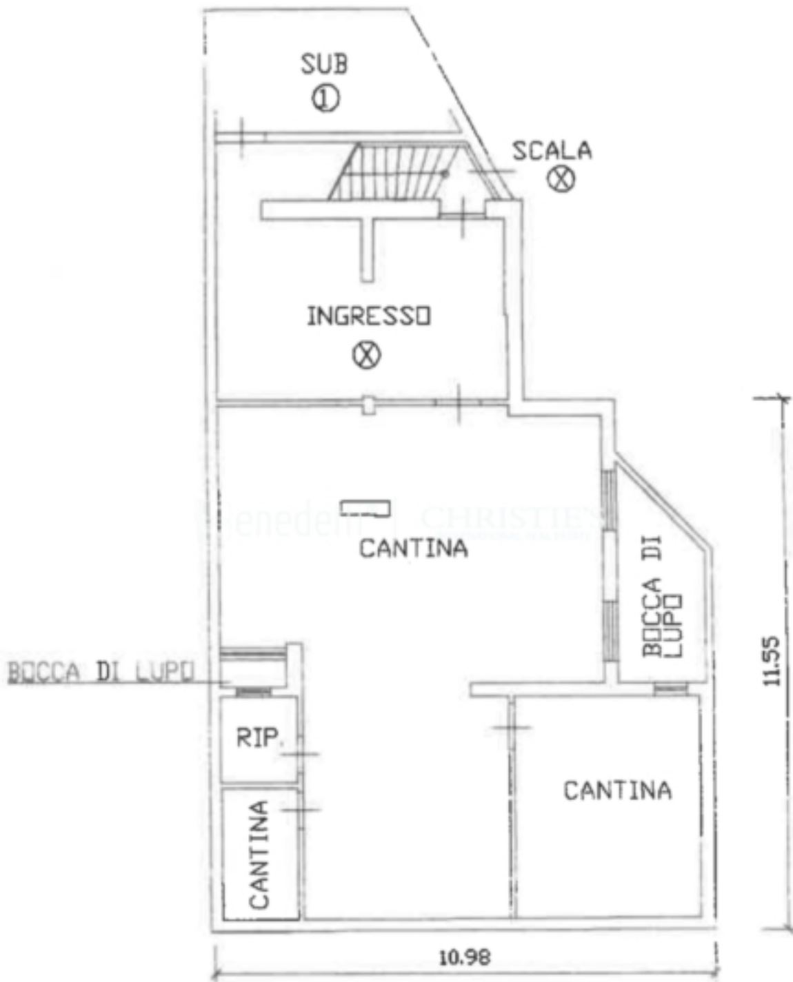
PIANTA PIANO CANTINA H=2.20-2.50m
